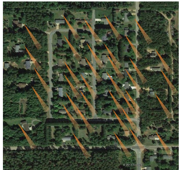
Figure 19. (Right) Picture of subdivision with homes served by private wells and septic system drainfields. Groundwater flow direction is from upper-left to lower-right. Orange shapes illustrate hypothetical plume paths downgradient of drainfields.
