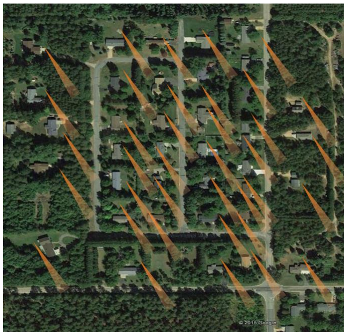
Figure 26. (Right) Picture of subdivision with homes served by private wells and septic system drainfields. Groundwater flow direction is from upper-left to lower-right. Orange shapes illustrate hypothetical plumes that septic system effluent travels downgradient of drainfields.
